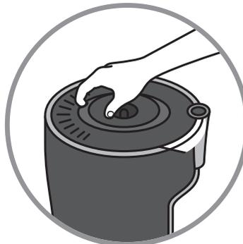
5. Remove separator by pulling straight out.
